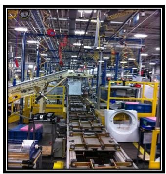
Use Tekno's own Non-synchronous Conveyor System for Palletized Product Assembly & Conveyance:
